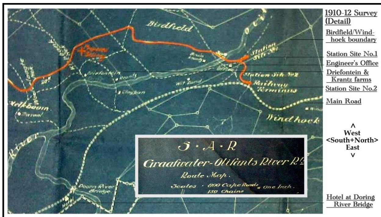
Illustration VII: Preliminary railway survey of 1910-1912 showing 2 alternative station sites
